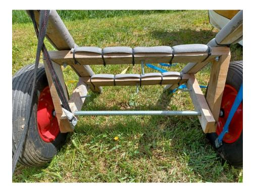
You need to drill two 20mm holes into the vertical elements in order to install the threaded axel. Screw with wood screws or angled braces the transversal elements on top of the vertical ones. Screw the longitudinal ones with normal screws and washers on top of the transversal ones. Use normal screws, as you'll need to remove them when folding the dolly.
