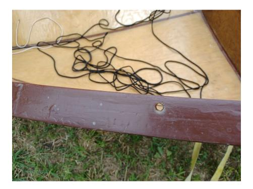
Measure your roof rack and see where the bars meet the gunwales. Drill the holes in that area. You can pass a rope or a nylon strap through each hole and tether the boat to the roof rack with it.
