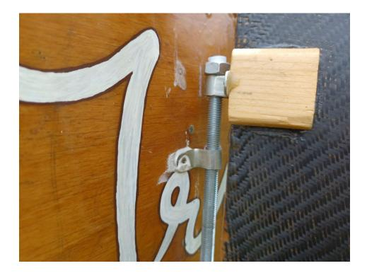
The omega braces need to have their correspondents on the outside of the transom. Screw and glue them to the transom in a way that will not change the rudder's position or overlap them. Remove the threaded rod, position the rudder then insert the rod again through all the omega braces. This is how the rudder will work.
