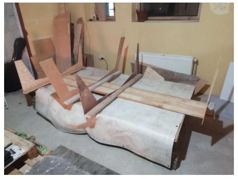
As such, make sure the bottom side is equally wide for all of them. If not one may sit higher or lower than the other. The outer sides of the molds are not so important. Leave them thick/wide enough to be strong.
