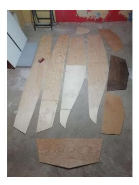
Pay particular attention when cutting the bottom panels out if you want to make Iris a sailor. You have to cut an extra notch in each panel, situated between the bulkheads. Through that notch will pass the central board. Subject to how thick you want your central board, you can make a combined width of the notches of 3 to 4cm (1.5 to 2cm on each panel).
