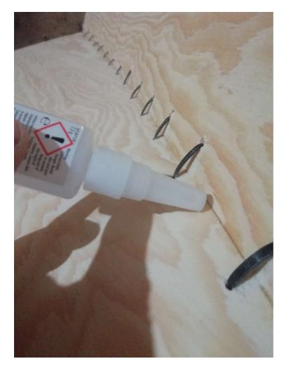
There may be areas where the ply panels are forced together by the zip ties. The glue will not hold them tight if the ties are removed. The gaps will simply crack open. In such a situation, keep one or two cable ties in place until the incoming epoxy operation will be fully cured. Remove the ties after. You may have to use plyers to pull on them, but mind the fact nylon will not bond with epoxy.
