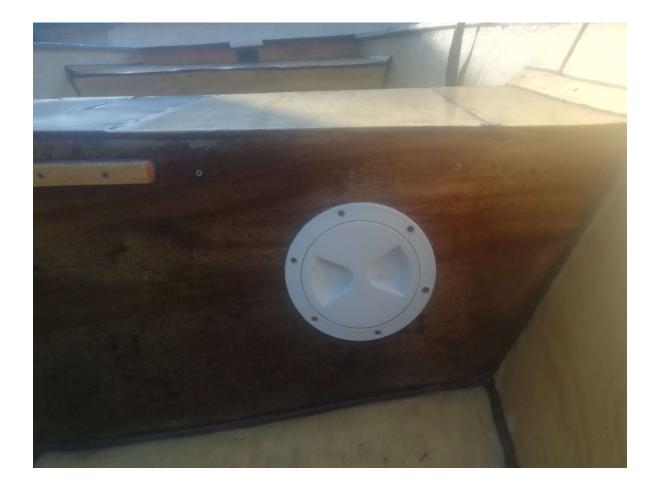
I used no frame for the bow box. The panels are small enough to take some weight, not to mention there will also be the mast step there, also taking some of the load.
