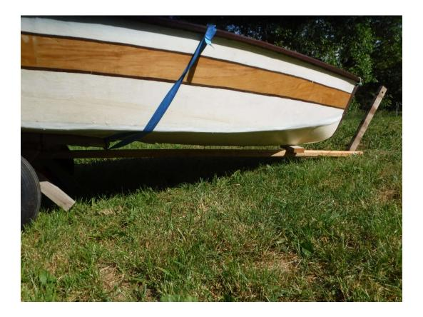
Secure the dolly under the boat with nylon straps passing through the tethering holes in the gunwales, otherwise the hull will slip and slide on top of it.
