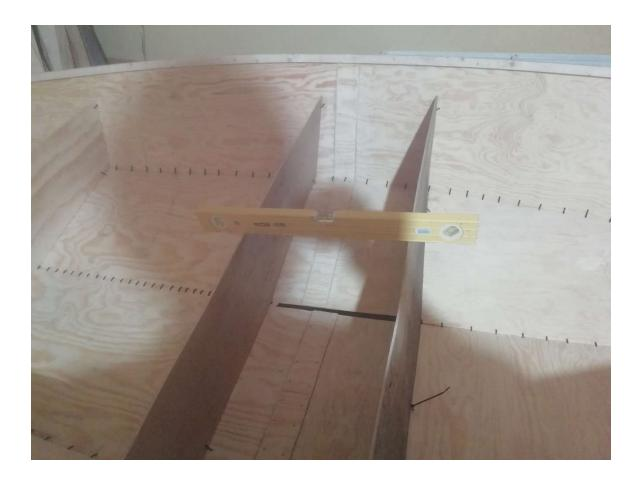
Its disadvantage is the complexity of the nesting operation and the use of 4 plywood sheets instead of 3. The plywood panels have to be cut in a way that their joint fits between the two bulkheads of the central thwart.
