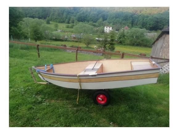
There are countless methods to build such a dolly. The internet is full of know-how. You can build out of PVC pipes, aluminum, iron pipes and wood. I made mine from wood as I had a lot of it around. I used a simple structural solution, which enables the dolly to be easily dismantled and folded (in order to fit in a trunk) or inside the boat.
