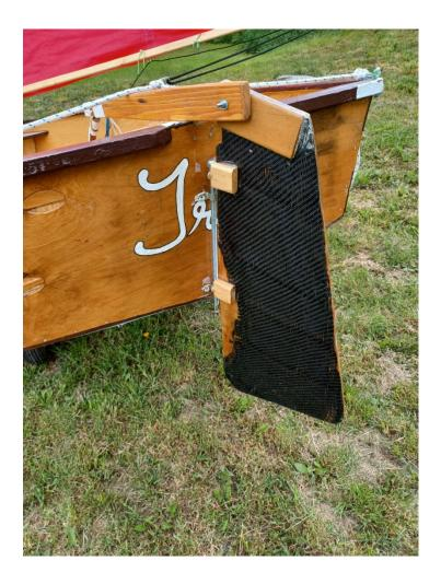
The lamination process is similar to the one used for the central board. For mine, I used some carbon fiber leftovers instead of glass.
