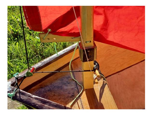
Drill 2x 6mm hole next to each other, 48cm above the foot of the mast. They will accommodate the line tethering the boom to the mast.
