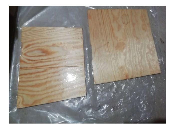
If you have time and a lot of sandpaper you can wait until the first coat is completely cured. Before applying the second, you'll have to sand the first with a 200-grit piece. The bondage between the layers will no longer be chemical, but mechanical. If the surface is left smooth, the next coat will not bond and will delaminate later.
