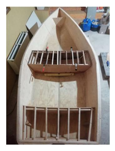
The bad part of the story is that I cannot give you any specific dimensions for the sticks. You have to measure the dimensions of the bulkheads and cut the sticks accordingly. I do not remember the distance between the vertical or the horizontal beams either. Just count how many of them are in the pictures and distribute them equally.
