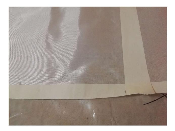
As the name says, these are very fine fibers of glass, technologically obtained through various processes (sometimes they also occur naturally). The fibers are then woven into meshes, fabrics or other products used in a variety of roles. What interests us the most are the ones used as a reinforcement agent for polymer products, like the one mentioned above.
