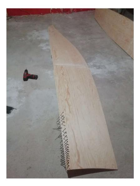
After having them in place you can start inserting the cable ties for the bottom panels. Do not tighten them yet. Just insert them into the holes and place the bottom panels onto the workbench. You can tighten them now. If inserting them after placing the panels on the bench, it will be more difficult to access them, as you may have to work under the boat.
