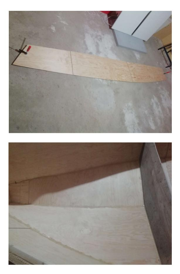
The second method involves making the joints invisible by masking them inside the central waterproof compartment. Being almost at the middle of the boat, this position has its advantages:
