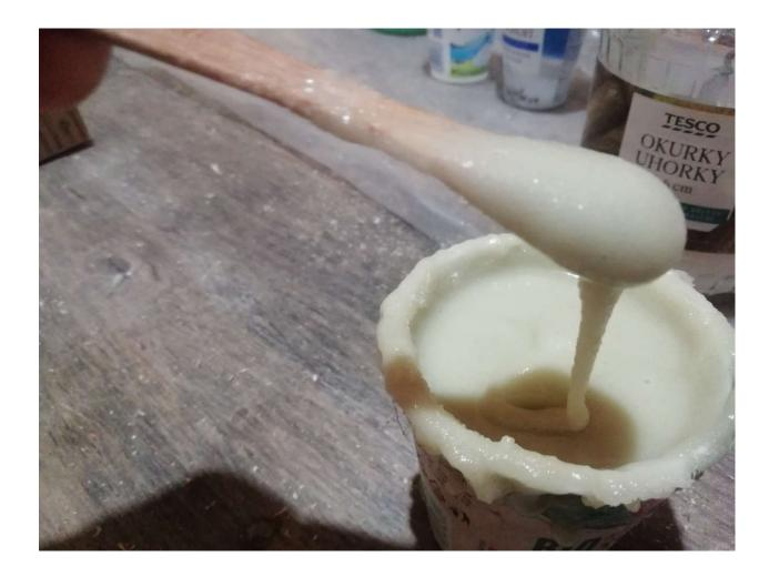
Making the filler will follow the exact steps as above, but you'll add a bit more flour to make the mixture even thicker. Do not exaggerate as you'll spoil everything. Do not oversaturate the resin with flour. The peanut butter comparison is not exaggerated, as that is the consistency you are aiming to obtain.
